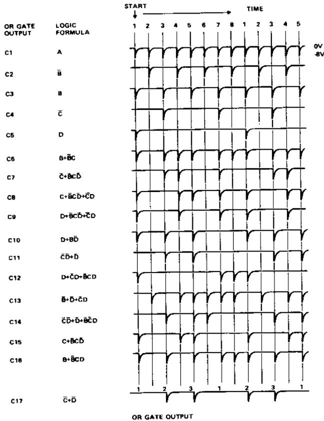
Fig. 2-29. OR gate output waveforms.
