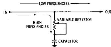
Fig. 2-5. High-cut tone-control circuit.
