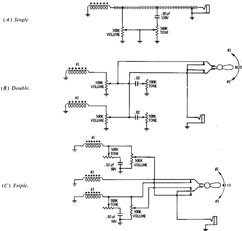
Fig. 2-4. Pickup circuits.
