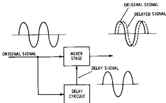
Fig. 2-14. Using signal delay to produce echoes.
